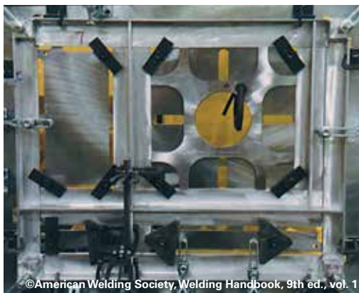
Welding fixture used to hold parts in position while welding
