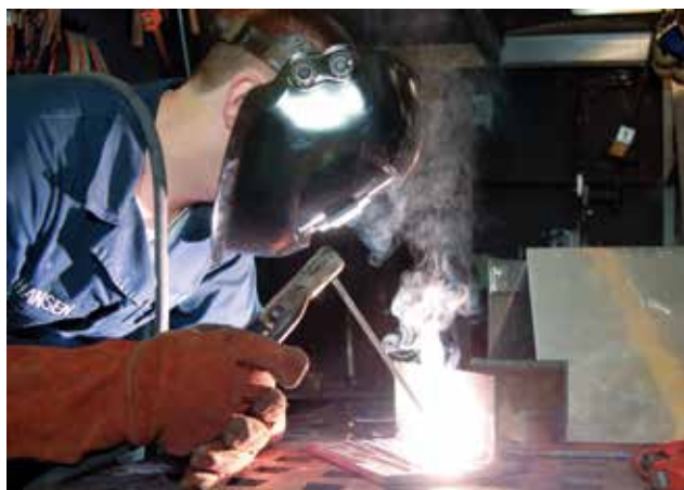
Welding beads with shielded metal arc welding
