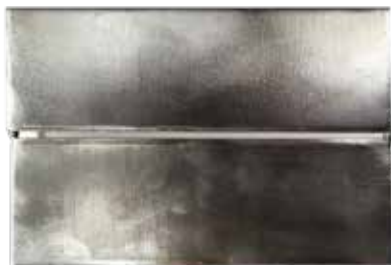
Tack welds at bottom ends of plate
