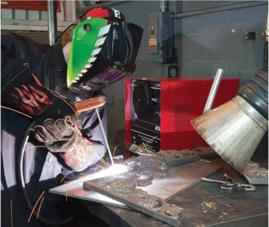
Welder using shielded metal arc welding
