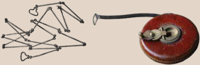
A Gunter's chain measured the wilderness of the United States. Chainmen laid out the chain and pulled on the handles to measure 66 feet.
