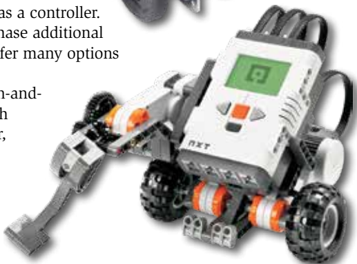
Robot constructed from a LEGO Mindstorms kit
