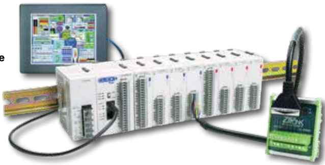
A PLC, or programmable logic controller
