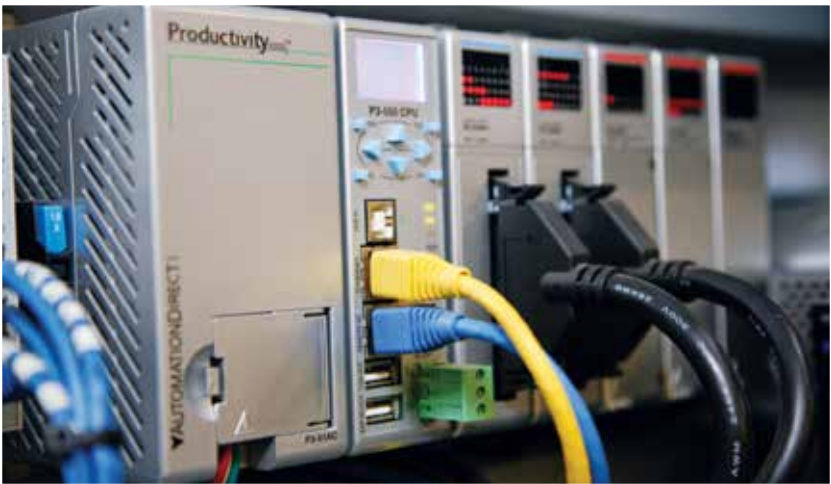
This programmable logic controller (PLC) controls motors and sensors . . . in this automated distribution plant.
