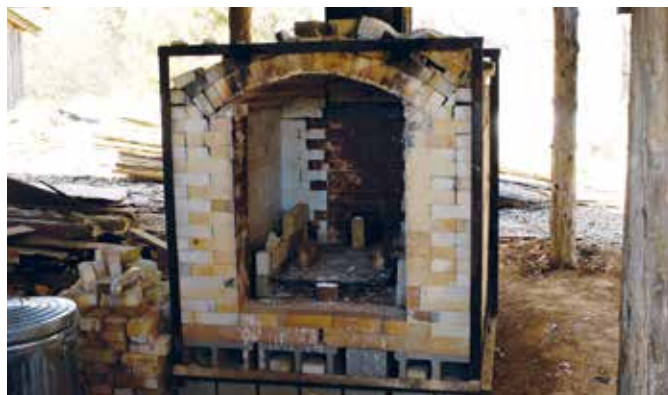
A typical fuel-burning kiln will take 12 to 24 hours to reach high-fire temperatures and another 24 hours to cool.
