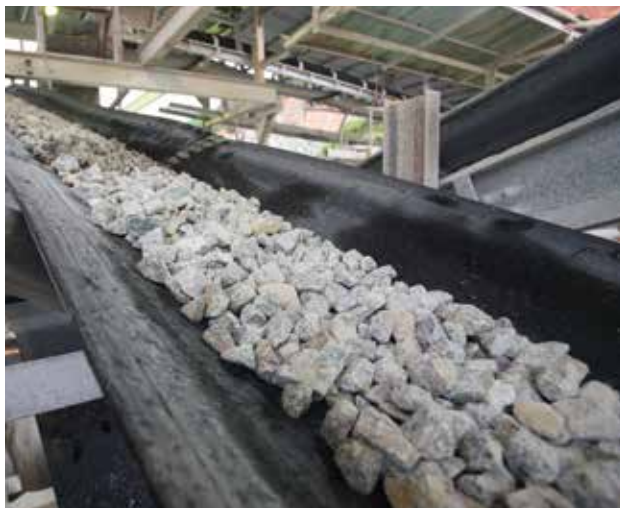
Crushed stone from primary crusher
