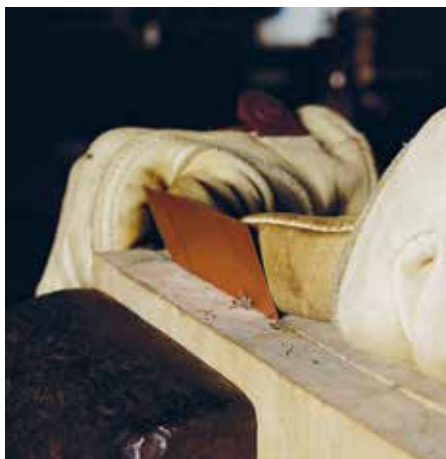
To demonstrate springback, use your hands to push the unworked metal into a 45-degree angle.
