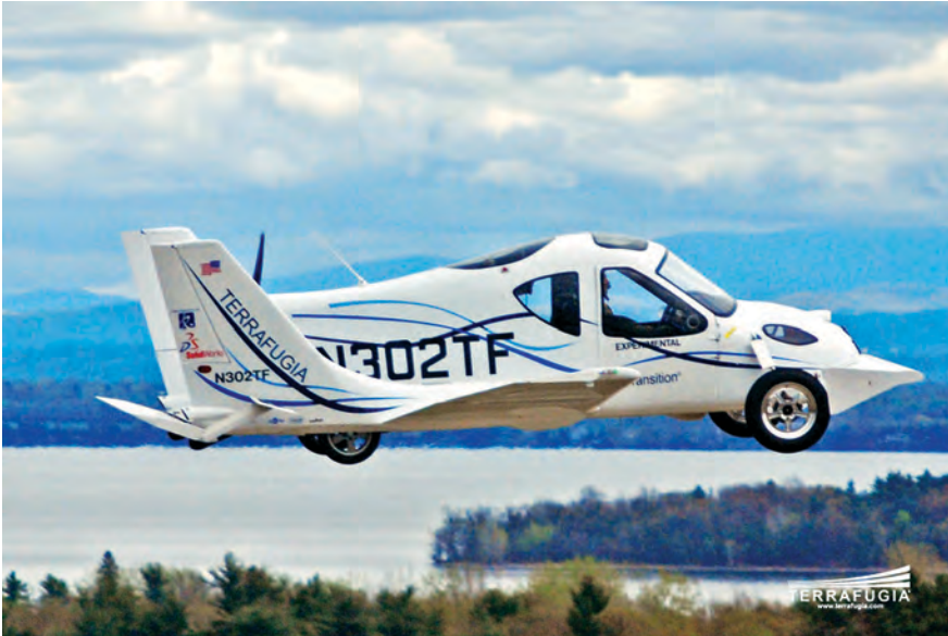
The Transition's folding wings are the unique invention that make it different from a flying car.
