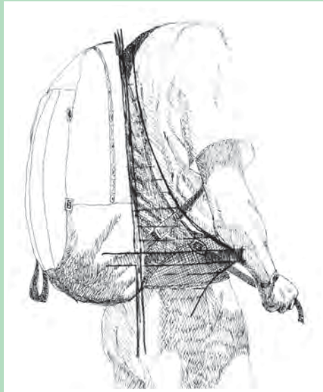
Fabel's EcoTrek™ backpack does not rely on shoulder straps to carry the load because it transfers much of the weight to the hips.
