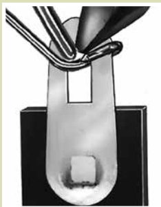
Apply solder to both the tip and the connection.
