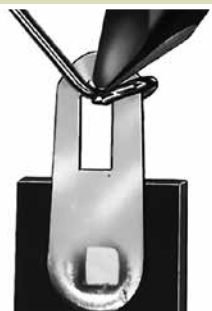
Heat the wire and the lug.
