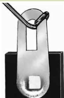
Attach the wire to a soldering terminal or soldering lug.
