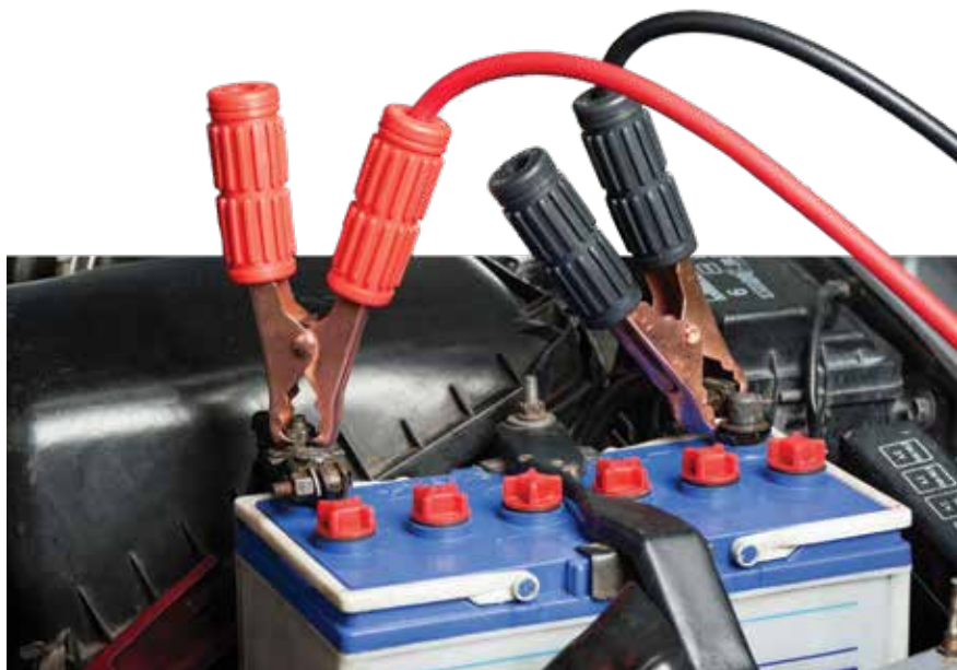
Correct jumper cable connections
