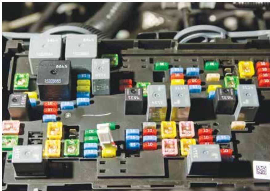
Typical fuse panel
