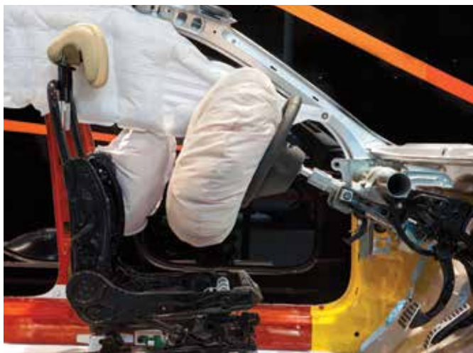
Air bags deploy automatically when a frontal crash occurs.
